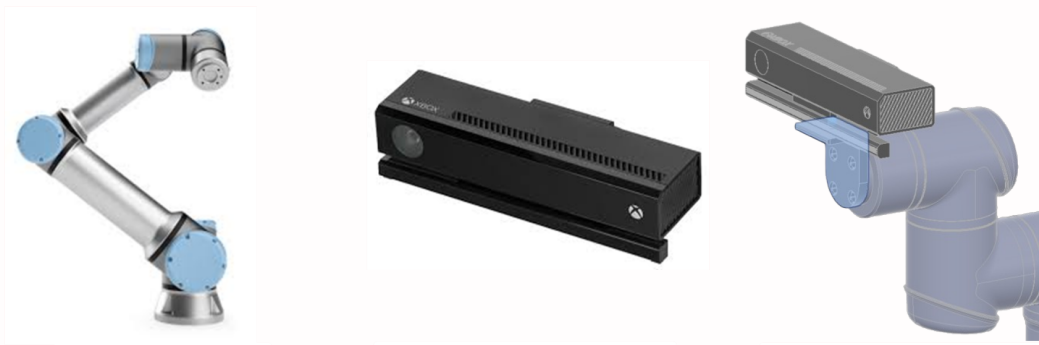
Figure 2: Hardware setup displaying the UR16e (left), the Kinect V2 sensor (middle), and a Fusion 360 visualization of the custom mount integrating both components (right).
